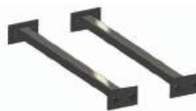
F14 Universal seat subframe to be adapted to the vehicle body floor according to FIA 253-65B Annex J instructions. - 2x 35 mm squared section pipes - 4x end plates (90x45) mm - 4x steel plates (110x65) mm - 4x M8 bushing RFST0079
