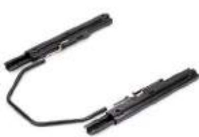
F3 Sliding tracks, travel 230 mm. No FIA. Z200002_A
